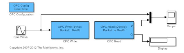
The OPC Config block defines the servers to use in the model, the pseudo-realtime behaviour of the model when it is simulated, and the actions to take when OPC-specific events occur (such as a pseudo-realtime violation, server shutdown, etc.)
